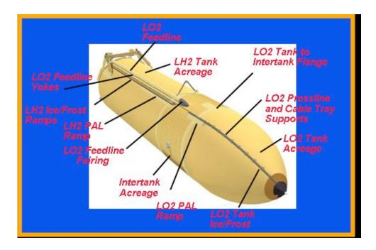
External Tank Thermal Protection System The project office is also investigating new techniques that will allow the foam to be inspected for internal defects without damaging it. The initial focus is on manually sprayed closeout, or final, foam applications. Although they are not yet fully developed, non-destructive evaluation techniques like backscatter radiography and terahertz imaging could offer an additional level of verification for the foam.
